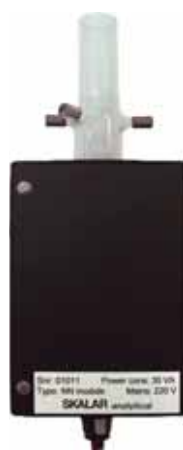
NO 2 and NO 3 Reactor
