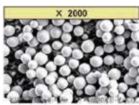
SEM of Hybrid particle
